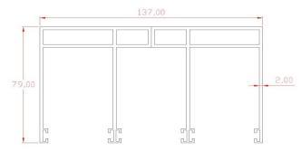
5-Rail profile cover: It is used to cover the idle parts inside the rail profiles..
