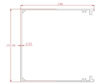
2-Engine box profile front cover: It is used to intervene the engine and working parts later.
