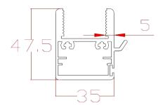
9-Non claw frame profile: It is used on the upper and lower parts of the guillotine glasses that do not attract each other. It is also used on the sides that do not pull.
