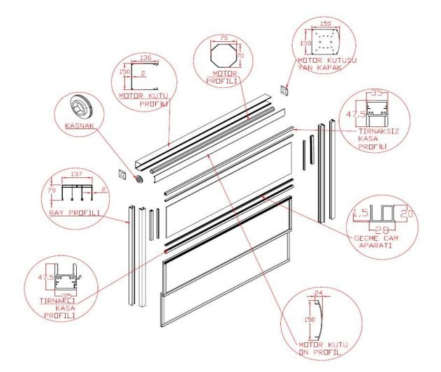
1-Motor box profile: It is used for motor and operating parts housing.
